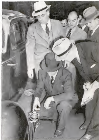
Clamped to the running board of a car involved in an accident, this handy unit checks up on its brakes
